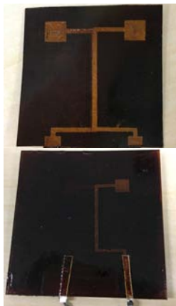
Figure 4: First prototypes: top) a prototype with a thin insulating layer, bottom) a prototype with a thick insulating layer.
